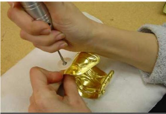
**Step Four:** The bracelet is shaped over a mandrel and the bezels are soldered on. The height of each bezel is adjusted by sanding the top.
