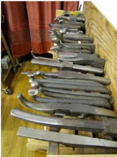
We need at least two hammers — one relatively light in weight, the other heavier. The light hammer is used for tracing and chasing, the heavy one for embossing or raising the relief. For small jewelry designs, especially in gold, I would recommend the use of chasing hammers # 22 and 26; for larger designs and/or hollow ware use #26 and #32, respectively.
