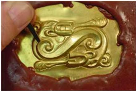
Tools should be made of the smallest appropriate size steel stock. The most commonly used sizes are those between 1/4 " and 1/8 " ( both round and square) cut into 4" to 4 1/2 " lengths. Shape the tool roughly on the 36 grit grinding wheel, then continue to work by files, 400 and 600 grit sand paper, and at the end polish with steel compound. Polishing will eliminate even the slightest imperfections.
