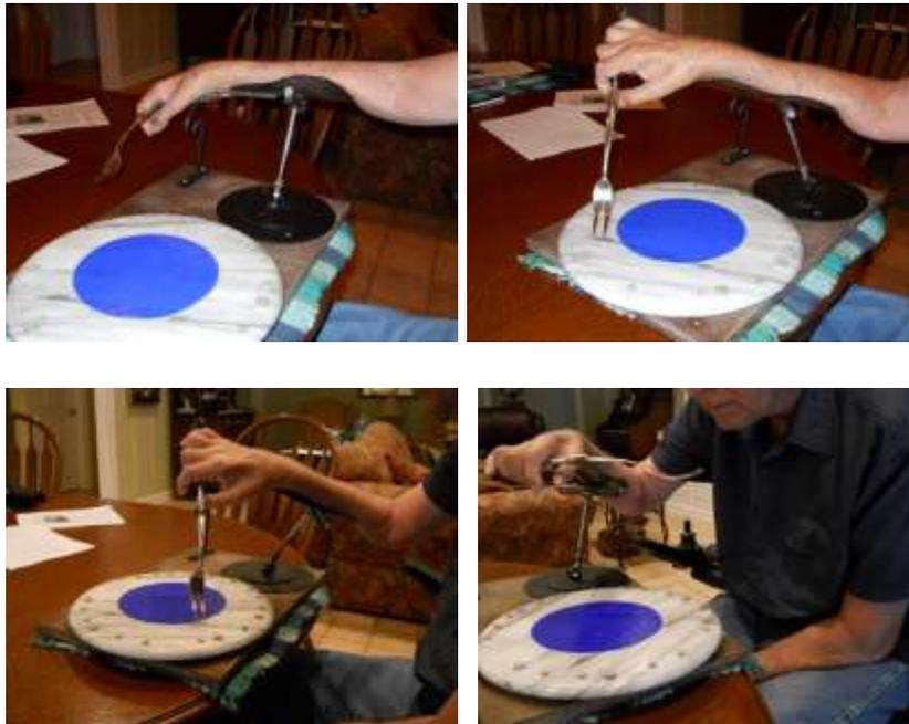
Note the position of the shaft and hinge as he rotates through the range of motion.
