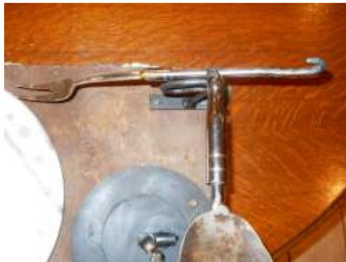
The next question was how do we attach the eating utensils? We wanted a way to be able to quickly attach a fork or spoon. Glen is right handed, so we decided to weld a ¼” socket extension to the left side of the Harbor Freight handle. On the other side we forged a “curl” to prevent his hand from sliding off the rest. These components are essential to form a hand rest and
