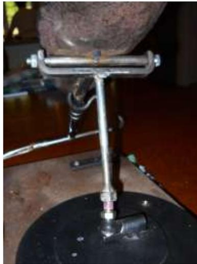
On top of the shaft we placed a sling shot shaped piece of 1/4 x 1/2 flat bar. There are holes drilled in each end to accommodate a 1/4” bolt. We then welded a piece of tubing or small pipe to the bottom of the arm rest. The arm rest is attached to the shaft by running the bolt through the sling shot and tubing to create a hinge.
